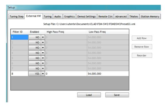
To enable another filter, for example the FBP20-1 filter for the 20m band, proceed as follows:
