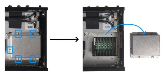
To close the FDM-S3 proceed in the opposite way, put back the filters shield and its screws, put back the top and bottom covers, put back the rear panel, tighten the screws and nuts of the SMA connectors.
