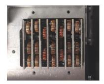
To decide which filter to use according to the tuned frequency, the FDM-SW2 software analyzes the configuration starting from slot number 1. It is therefore important to **insert the bypass in the last slot used** to have it chosen as the reception path if no other filter is enabled for the current tuning frequency.
